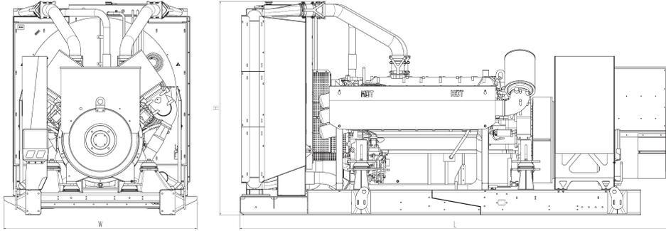
Drawing above for illustration purposes only, based on a standard open power 400 Volt engine-generator set. Lengths may vary with other voltages. Do not use for installation design. See website for unit specific template drawings.
