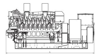
Drawing above for illustration purposes only, based on a standard open power 400 Volt engine-generator set. Lengths may vary with other voltages. Do not use for installation design. See website for unit specific template drawings.
